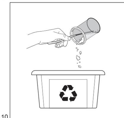
After the water has been emptied from the cartridge, remove any dirt and microfibres from inside the cartridge and dispose of it in DRY general waste. A paper towel can be used to collect as much material as possible.
