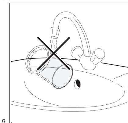
To preserve the positive impact of the filter on the environment, avoid the use of water to clean the filter cartridge. Instead, throw away the waste collected by the filter cartridge in the general dry waste (avoid dispersion of plastic fibre in water ambient).
