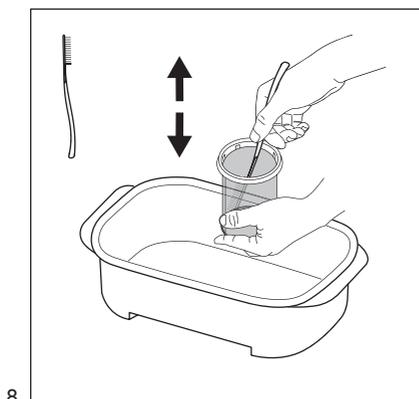
Holding the cartridge inside the container, use the brush-spatula tool available in the filter box. With up/down brush movement remove as much as possible the fibres attached to the cartridge net to help the evacuation of water.
