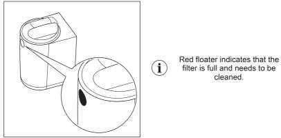
In **"red alarm"** mode (when the floater is activated) the filter will not stop the washing cycle, but it will work in a bypass mode and will not filter anymore.
