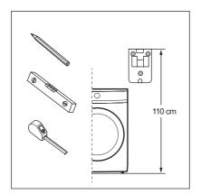
2. The position of your filter needs to follow these listed points (a and b): a. Position the wall support at the correct height, measuring 110 cm\* from top of the wall support to the floor (or pedestal if present). \*Tolerance admitted in filter height position is +/-5 cm.
