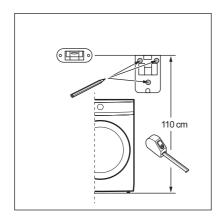
b. Use a level to check that the 3 drilling punches are level and well-aligned before drilling.
