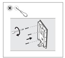
4. Attach the wall support with the screws and plastic anchors provided, making sure it is straight and securely affixed to the wall.
