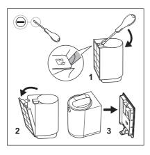
1. Remove the filter from packaging box and remove the wall support with the help of a flat screwdriver.
