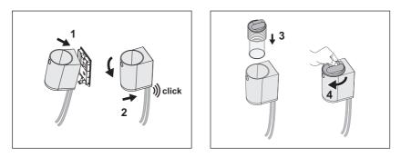
Before proceeding to the next topic Daily use & care and cleaning, start the short washing programme and follow it until the end. Be sure that no leakages appear from the filter and its connections. In case of water leakage, proceed as described in paragraph 8. Detach the filter assembly from the wall support and tighten the collars. To reinstall the filter, repeat the steps in paragraph 7.
