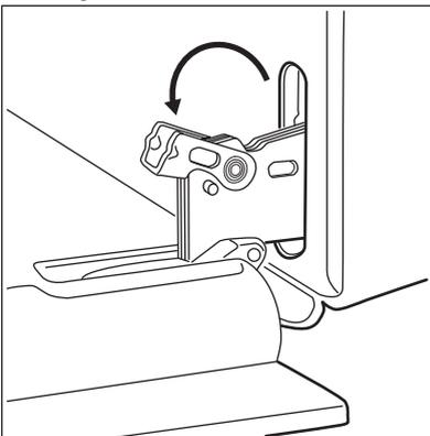
3. Close the oven door halfway to the first opening position. Then pull forward and remove the door from its seat.
