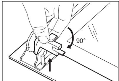
7. First lift carefully and then remove the glass panel.
