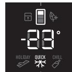
Use the quick freeze mode when you add a large amounts of food to the freezer compartment. The freezer compartment temperature will show -23°C. (This temperature cannot be changed while pressing the "Modes" button to select quick freeze will now operate for 90 minutes then switch to normal operation.)
