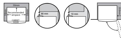
NOTE: In installation where both sides and the rear of the refrigerator are not enclosed by cabinetry eg the refrigerator is placed against a wall, the clearance between the rear of refrigerator and the wall should not be greater than 75mm.
