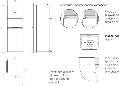
If you do not have a cupboard with allowance for air flow above the refrigerator, the recommended clearance area on top increases to 90mm.
